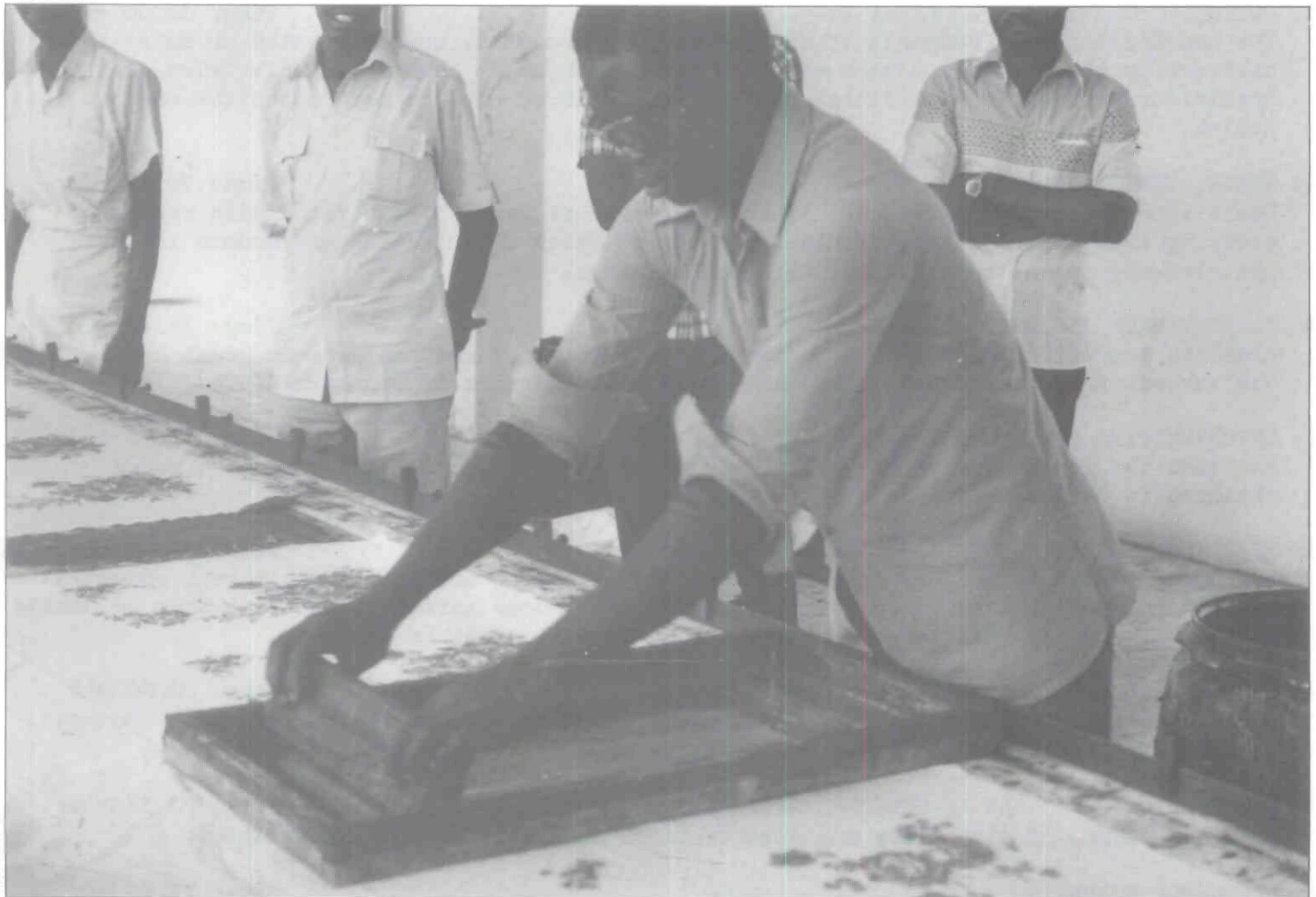
Silkscreen printing at a textile factory in Khartoum. This can easily be adapted to a cottage-industry at village level.
